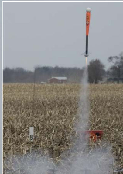
Pop Fly Estes kit by Zachary Fisher powered with a B4. A ball sits on the bat shaped rocket and free falls after apogee and the "bat" has a streamer.
